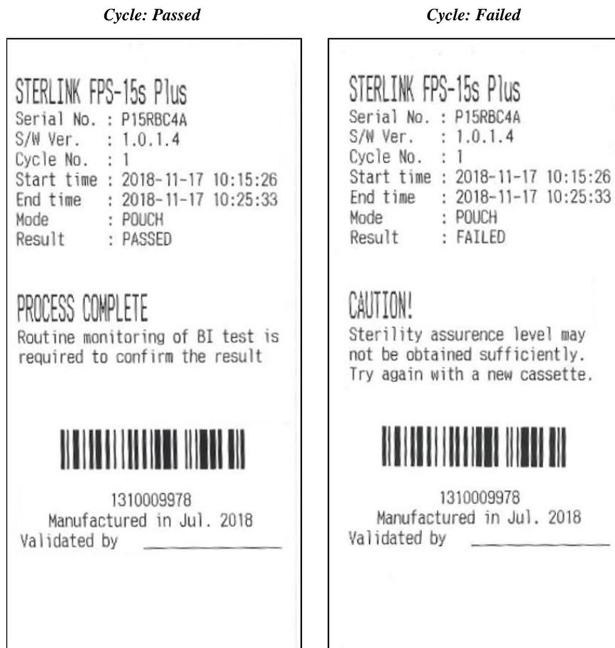
**Figure 7.2 Short format report for passed and failed cycle**
